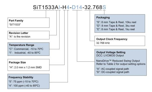
The following examples illustrate how to select the appropriate temp range and output voltage requirements:
