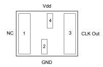
Figure 1. Pin Assignments
