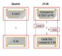
Figure 3. JYJE1533 Footprint Compatibility with Quartz XTAL Footprint<sup>[6]</sup>
