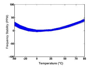
Figure 8. Frequency Stability over Temperature
