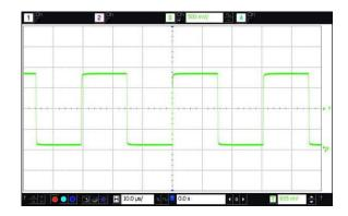
Figure 14. LVCMOS Output Waveform (Vswing = 1.8V, JYJE1533AI-H4-DCC-32.768)
