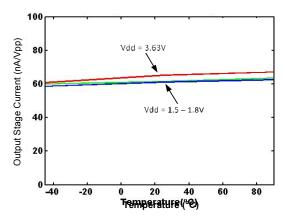
Figure 10. Output Stage Current Over Temperature
