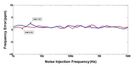
Figure 12. Power Supply Noise Rejection (±150mV Noise)
