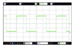
Figure 6. LVCMOS Waveform (Vdd = 1.8V) into 15 pF Load
