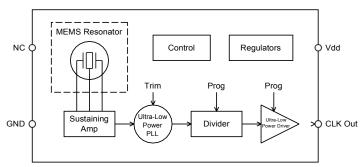
Figure 2. JYJE1533 Block Diagram
