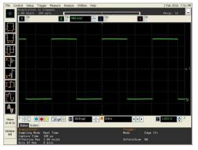
Figure 3. LVCMOS Output Swing (Vdd=1.8V)
