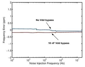
Figure 4. Power Supply Noise rejection (PSNR)
