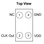
Figure 1. Pin Assignment
