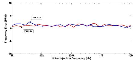
Figure 9. Power Supply Noise Rejection (±150mV Noise)
