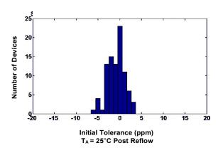
Figure 5. Initial Tolerance Histogram
