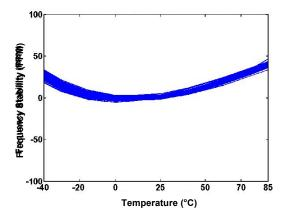
Figure 6. Frequency Stability Over Temperature
