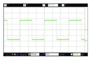
Figure 10. LVCMOS Output Waveform (Vswing = 1.8V, JYJE1630AI-H4-DCC-32.768)
