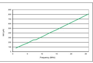
Figure 9. Idd vs Frequency with 10pF load
