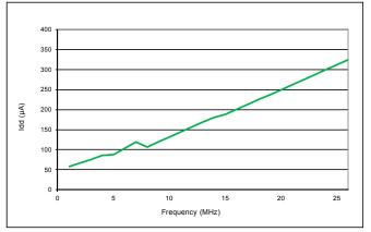
Figure 8. Idd vs Frequency without load
