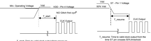
T\_start: Time to valid clock output from power on
