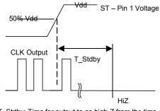
T\_Stdby: Time for output to go high-Z from the time ST pin crosses 50% threshold
