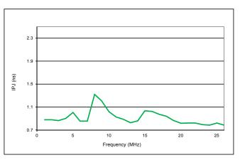
Figure 13. RMS Phase Jitter Random vs Frequency<sup>[8]</sup>
