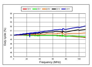
Figure 11. Duty Cycle vs Frequency
