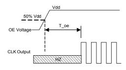
T\_oe: Time to re-enable the clock output
