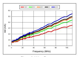
Figure 8. Idd vs Frequency
