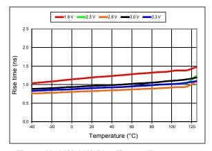
Figure 12. 20%-80% Rise Time vs Temperature
