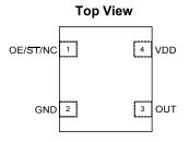
Figure 1. Pin Assignments
