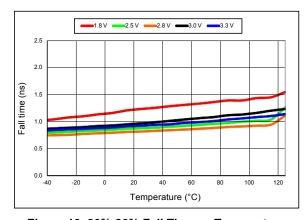
Figure 13. 20%-80% Fall Time vs Temperature
