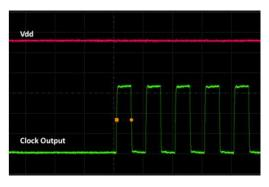
Figure 18. Startup Waveform vs. Vdd (Zoomed-in View of Figure 17)
