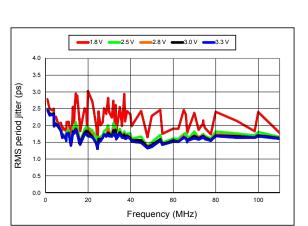
Figure 10. RMS Period Jitter vs Frequency
