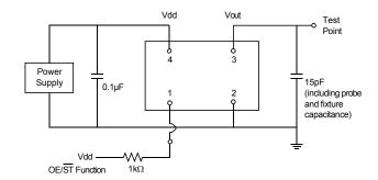
Figure 2. Test Circuit
