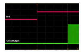
Figure 17. Startup Waveform vs. Vdd
