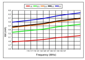
Figure 8. Idd vs Frequency
