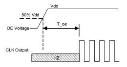
T\_oe: Time to re-enable the clock output
