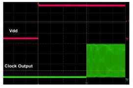
Figure 17. Startup Waveform vs. Vdd
