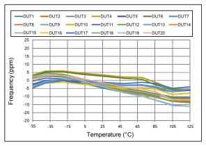
Figure 9. Frequency vs Temperature
