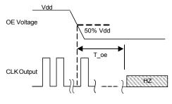
T\_oe: Time to put the output in High Z mode
