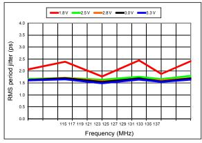
Figure 10. RMS Period Jitter vs Frequency
