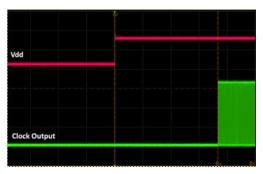
Figure 17. Startup Waveform vs. Vdd
