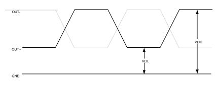
Figure 2. LVPECL/HCSL Voltage Levels per Differential Pin (OUT+/OUT-)
