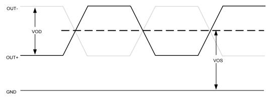
Figure 4. LVDS Voltage Levels per Differential Pin (OUT+/OUT-)
