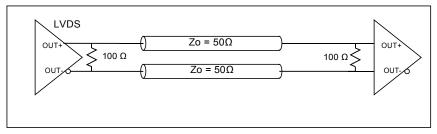
Figure 14. LVDS double DC termination
