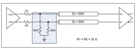
Figure 15. HCSL interface terminatio
