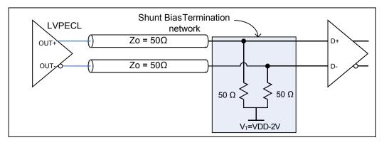
Figure 11. LVPECL with DC-coupled parallel shunt load termination
