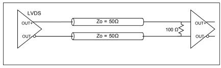
Figure 12. LVDS single DC termination at the load
