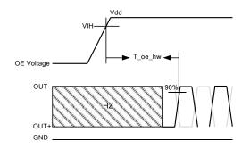
Figure 6. Hardware OE Enable Timing
