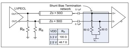
Figure 8. LVPECL with AC-coupled termination
