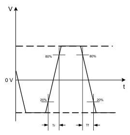
Figure 5. LVDS Differential Waveform
