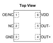
Figure 1. Pin Assignments
